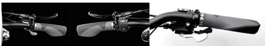
When braking hard by pulling the brake levers towards the handle bars, you should not push the braking force to its upper limit. Or, the braking distance will be extended and there is a risk of accident. Adjust the brake levers as mentioned above.
